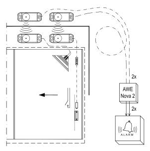
The "AWE Nova" evaluation module can be used with existing installations as a replacement product for the discontinued IDENTLOC system. This evaluation unit detects the IDENTLOC sensors automatically and evaluates the status thereof. The Honeywell sensors can be connected to sensor input 1 and 2, and now also be evaluated independently.
