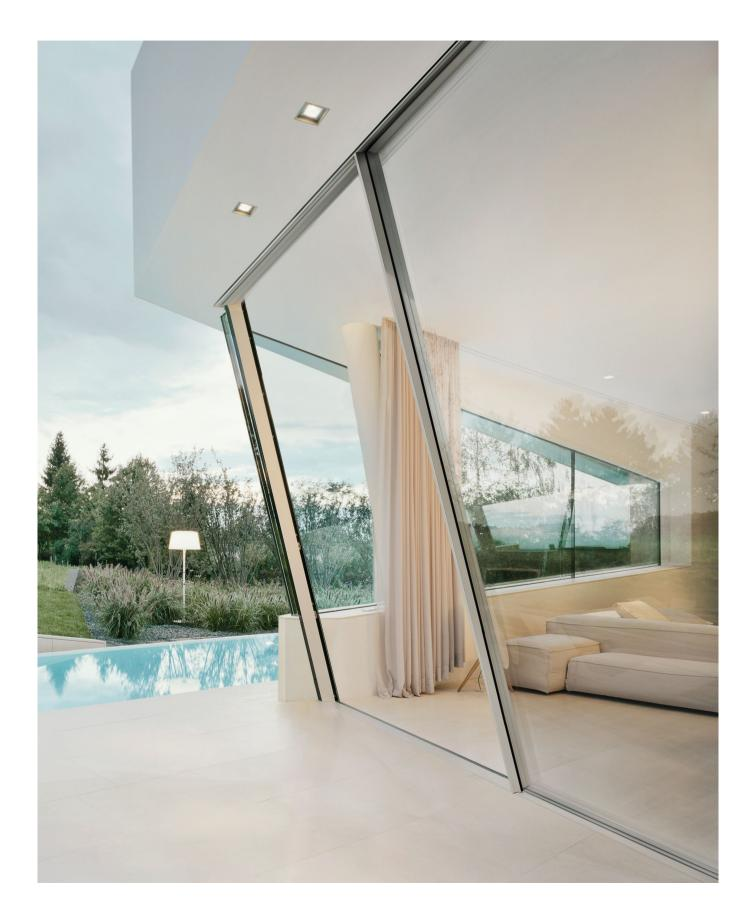
Sky-Frame Slope sliding doors can either extend into the room or project outwards from the facade at an angle of up to 20°. The system creates a distinctive spatial geometry while meeting all Sky-Frame standards. The bearing assembly accommodates all vertical and horizontal forces, thereby achieving superior running performance. Regardless of the direction of the door, the drainage system meets all requirements for driving rain resistance.
